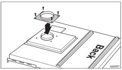
■ Mount the vent collar on the rear of the ventilation system.
